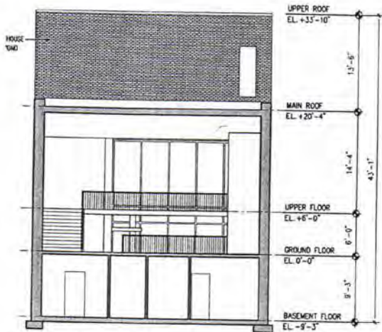
East West Section at Ground Floor
